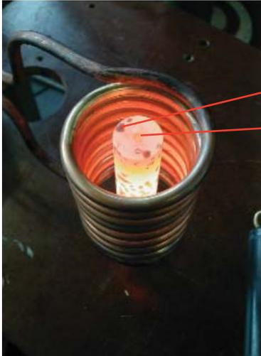
Heating the steel to over 900°C in the presence of oxygen leads to the formation of scale.
