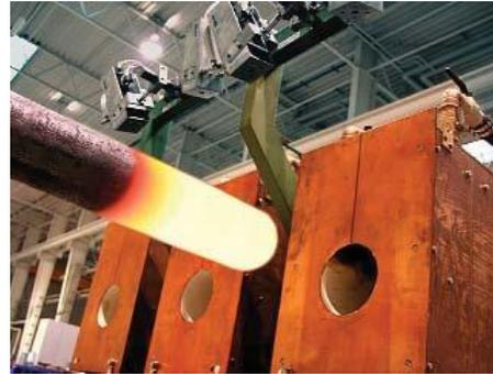
The Metis MS09S provides clear advantages over conventional pyrometers in this case. Changes in surface emittance affect the measurement significantly less.
