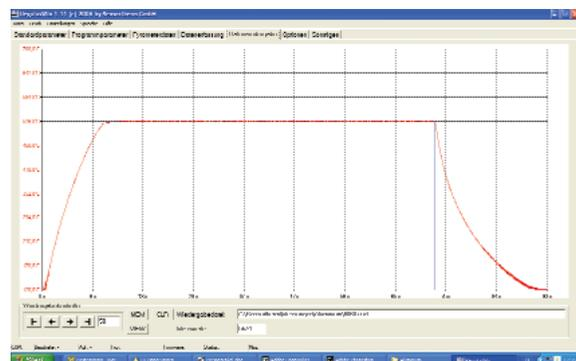
**Example:** Induction hardening of aluminum at 525°C, Regulus in combination with a Metis MI18 pyrometer
