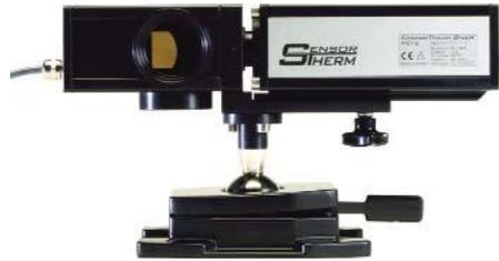
Adding an SC10 scanning mirror allows the pyrometer optical path to be continually diverted. In this way the extremely small field of view of the Metis pyrometer can locate even the slightest occurrence of scale and is able to display the true temperature by means of the integrated maximum-value storage. The SC10 scanning mirror is also excellent for measurements on small diameter wires.
